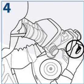
4 Rotate the focusing knob to bring the specimen into focus
