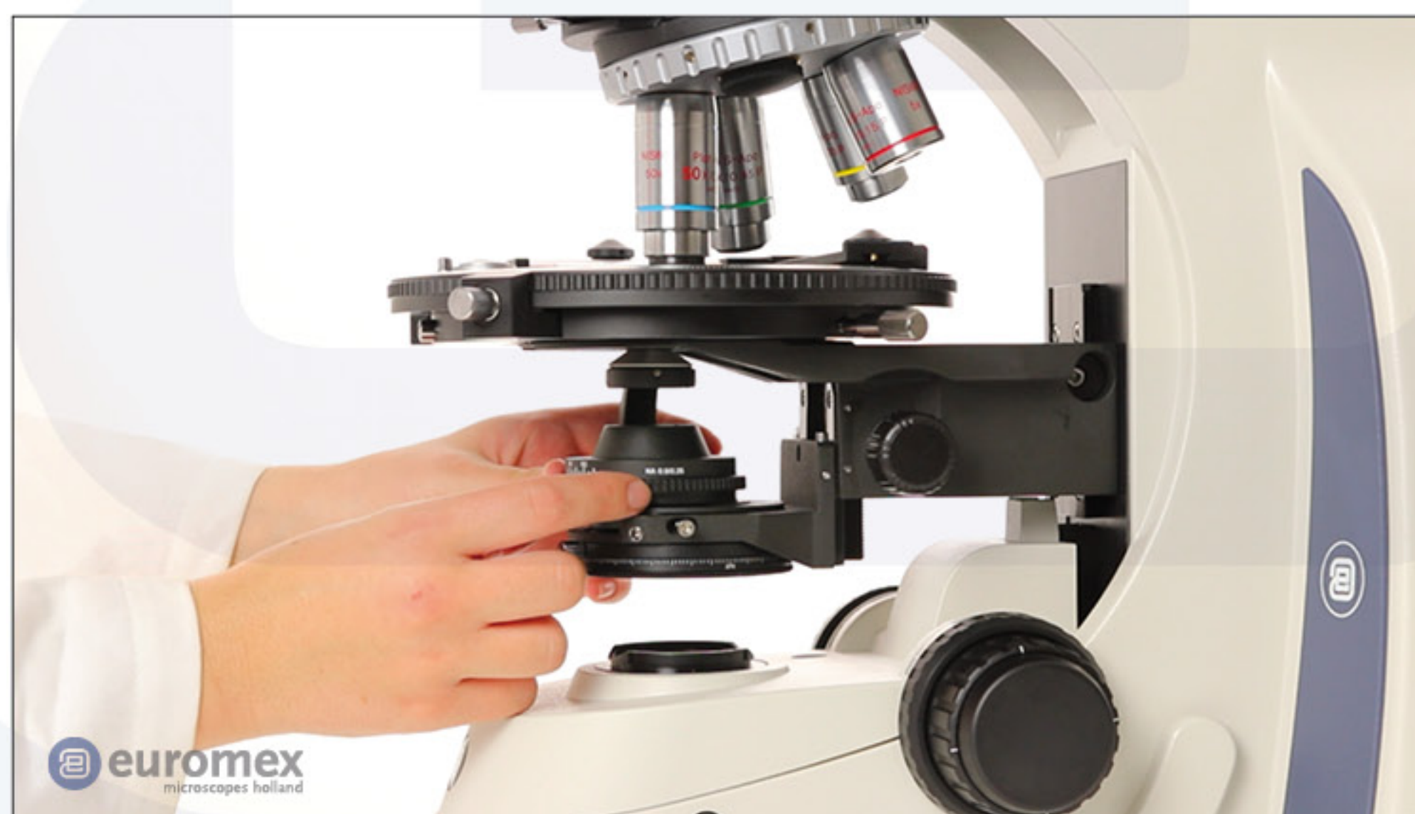
Turn the stage holder up and the condenser holder down
