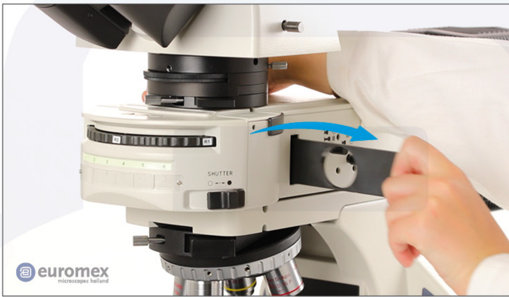
First remove the dust protection and insert the polarizer
