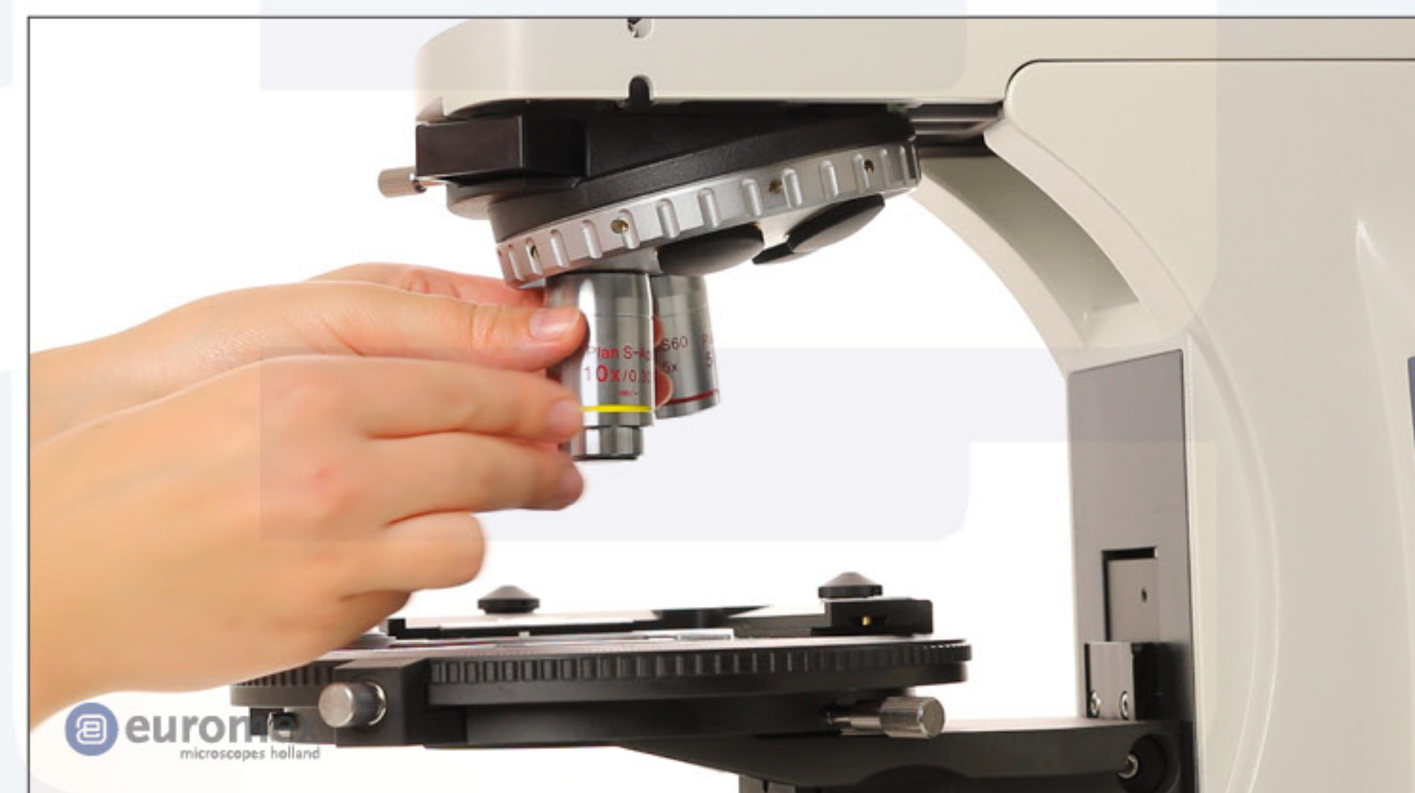
Turn the nosepiece to the left to access the next position Install the 10x, 20x, and 50x objectives in the same way
