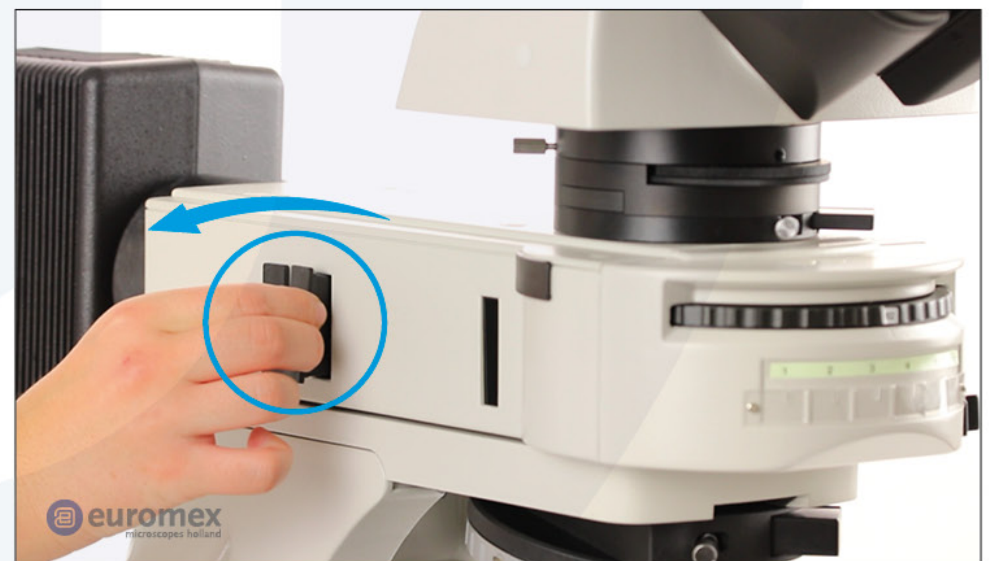
To use the supplied color filters, first remove the dust protection
