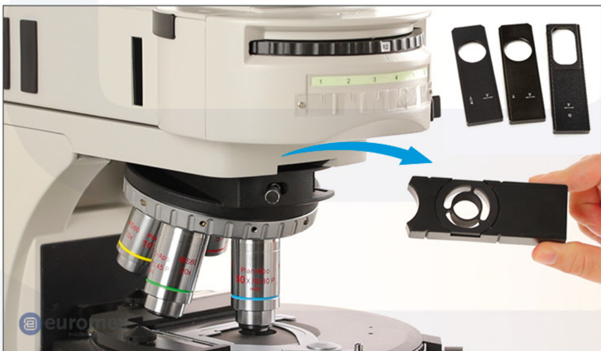
To use the supplied compensation plates, first remove the dust protection
