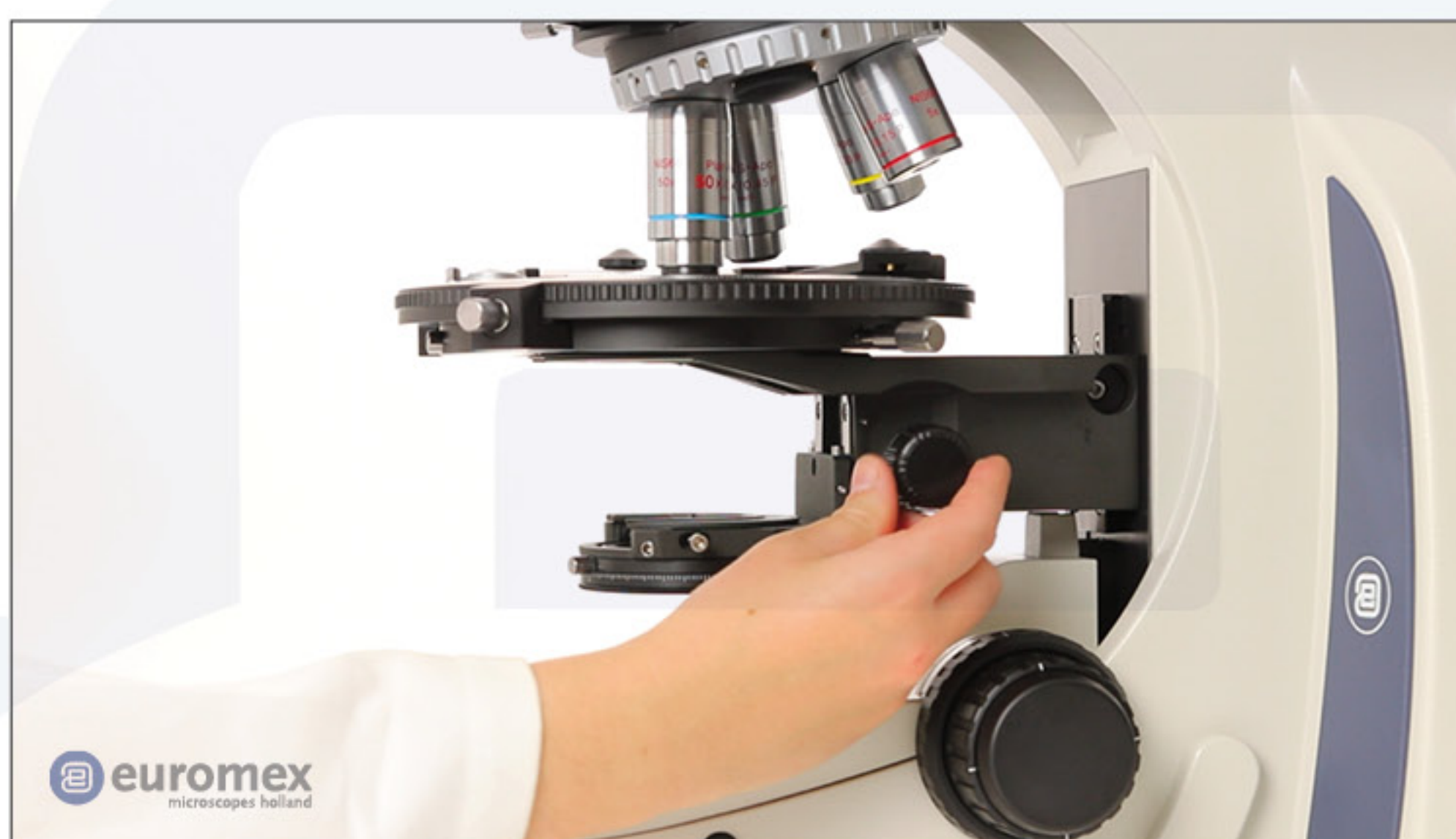
Turn the stage holder up and the condenser holder down
