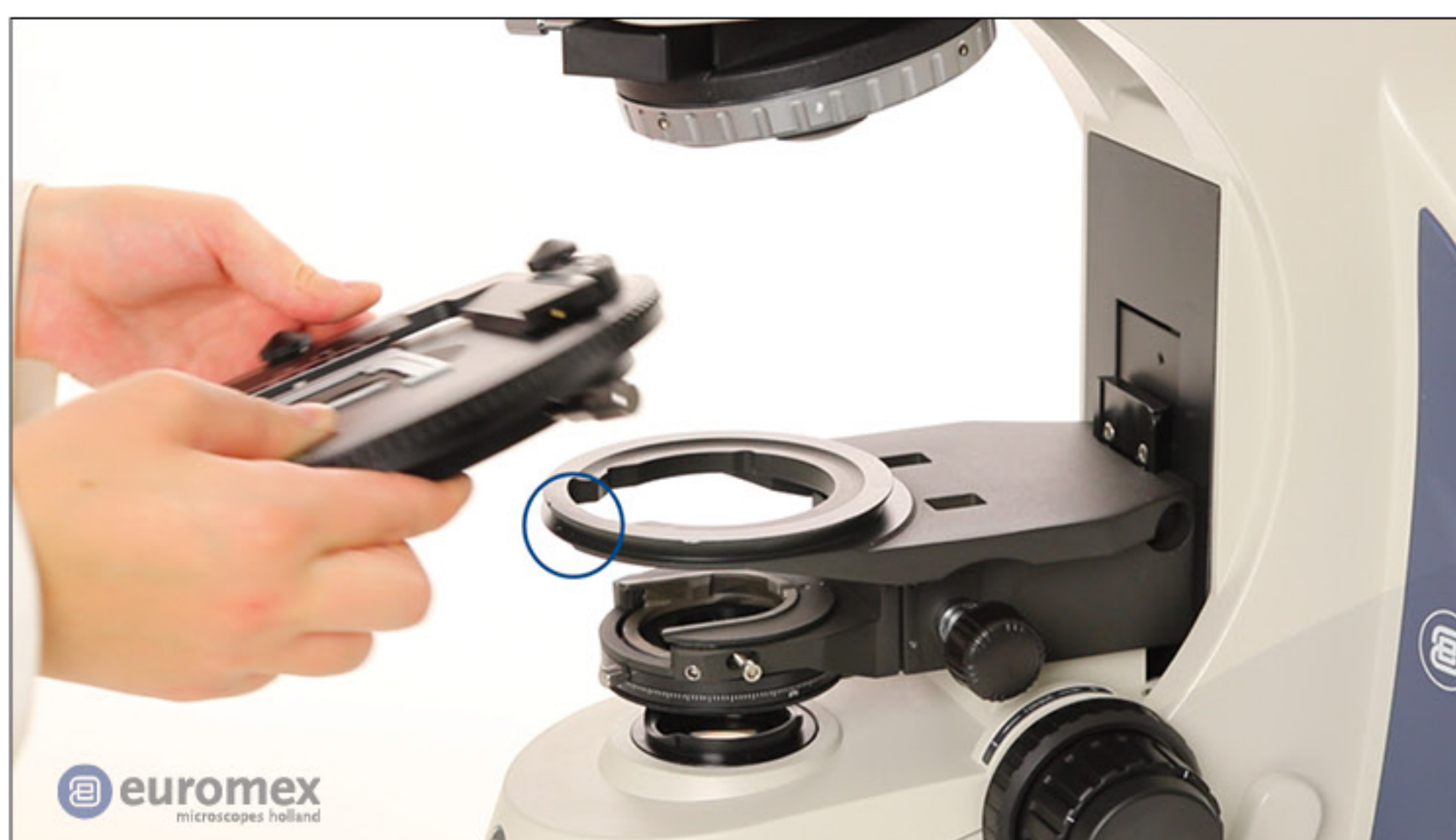
Attach the stage in the correct position
