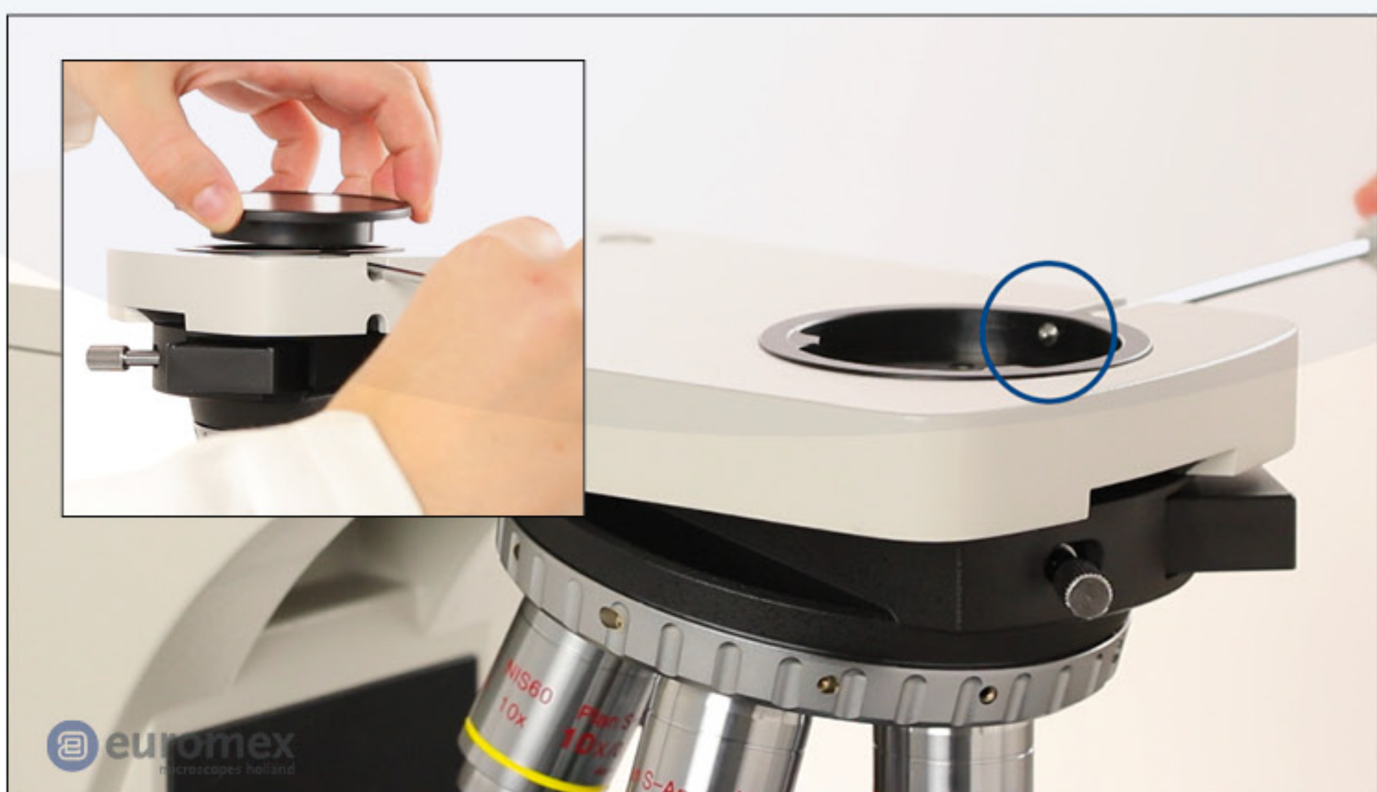
Remove the dustcover plate. Make sure that the screw does not block the installation of the component
