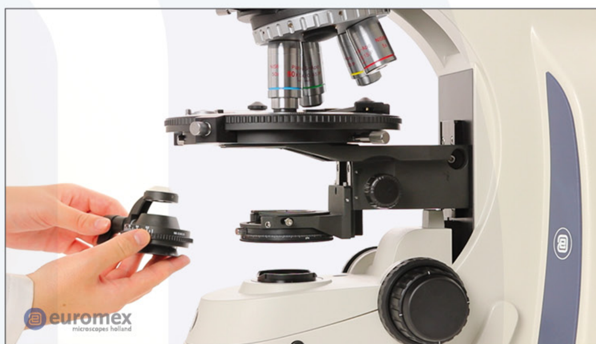
Insert the condenser into the condenser holder
