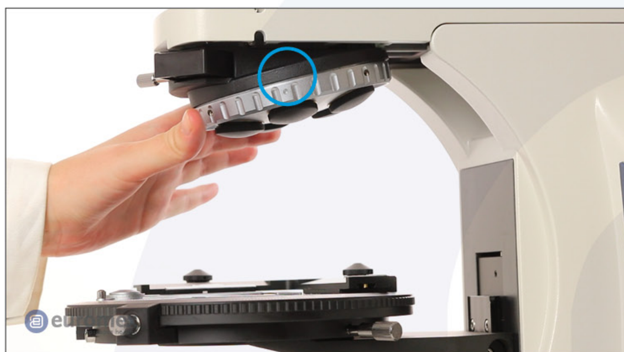
Note the indicated position (indentation) where the 5x objective should be installed
