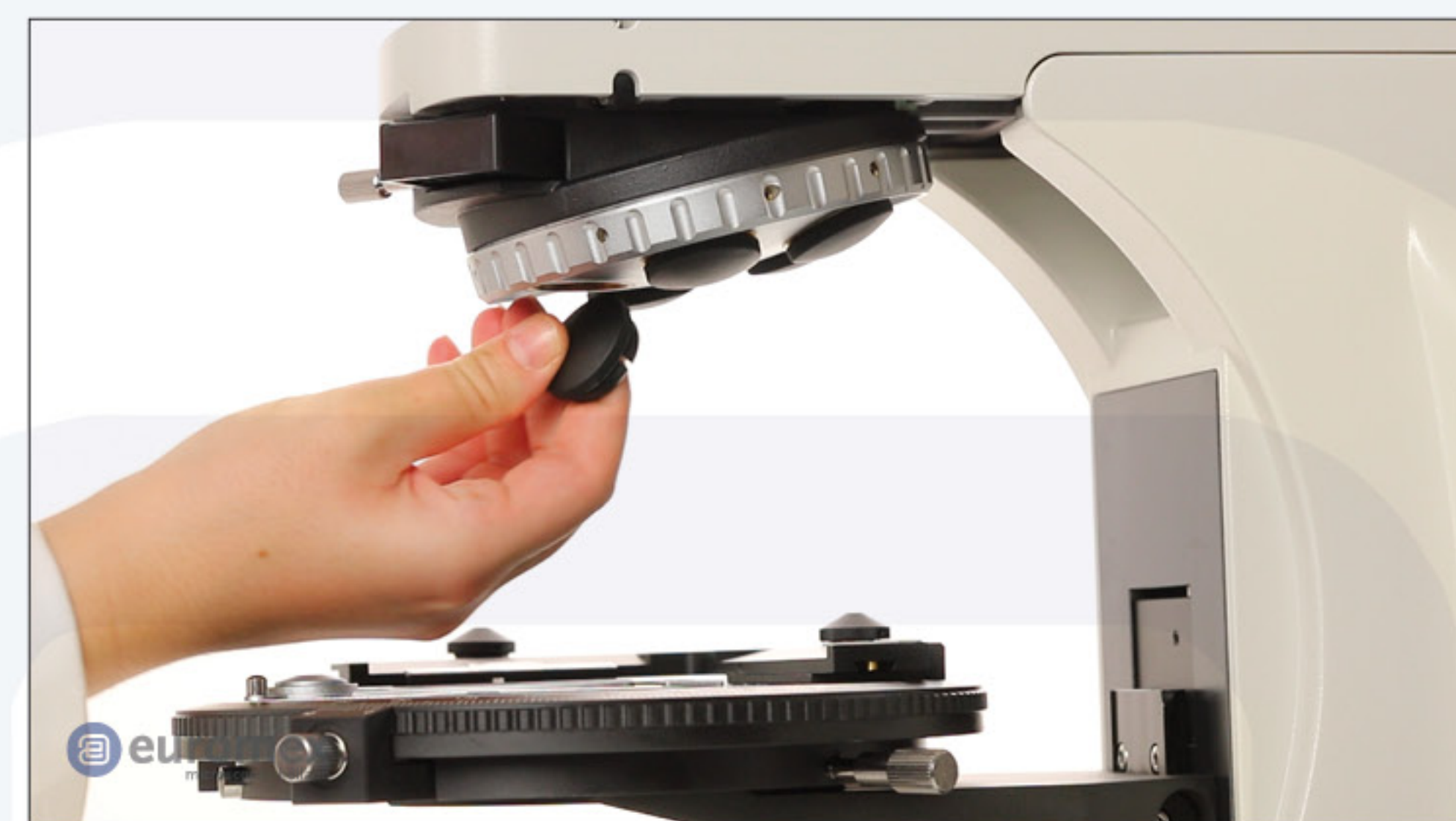
Remove the objective thread dust caps
