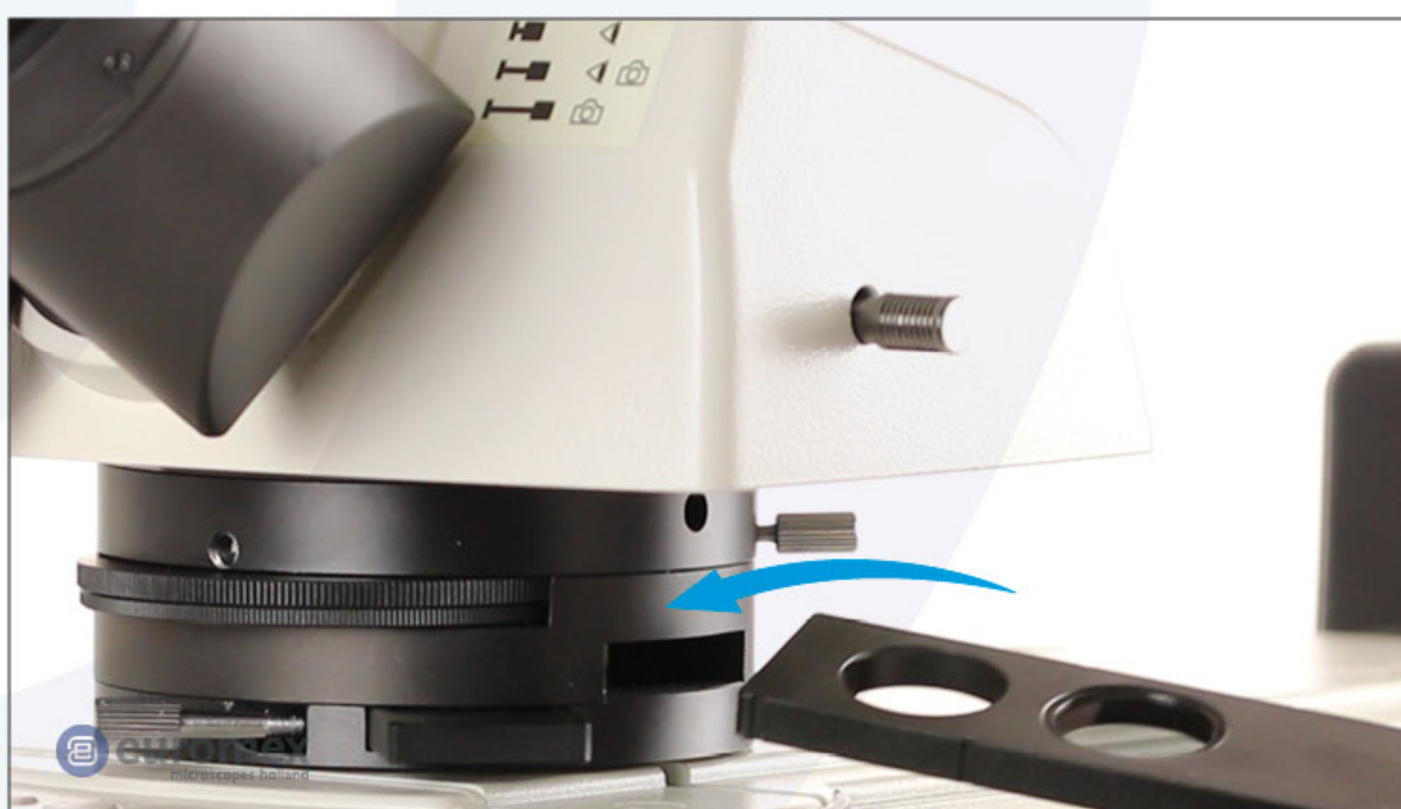
Insert the analyzer
