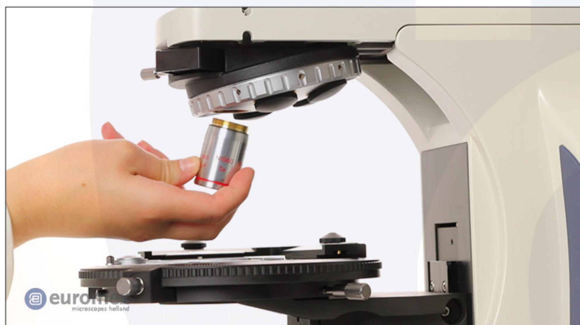
Screw the 5× objective into place
