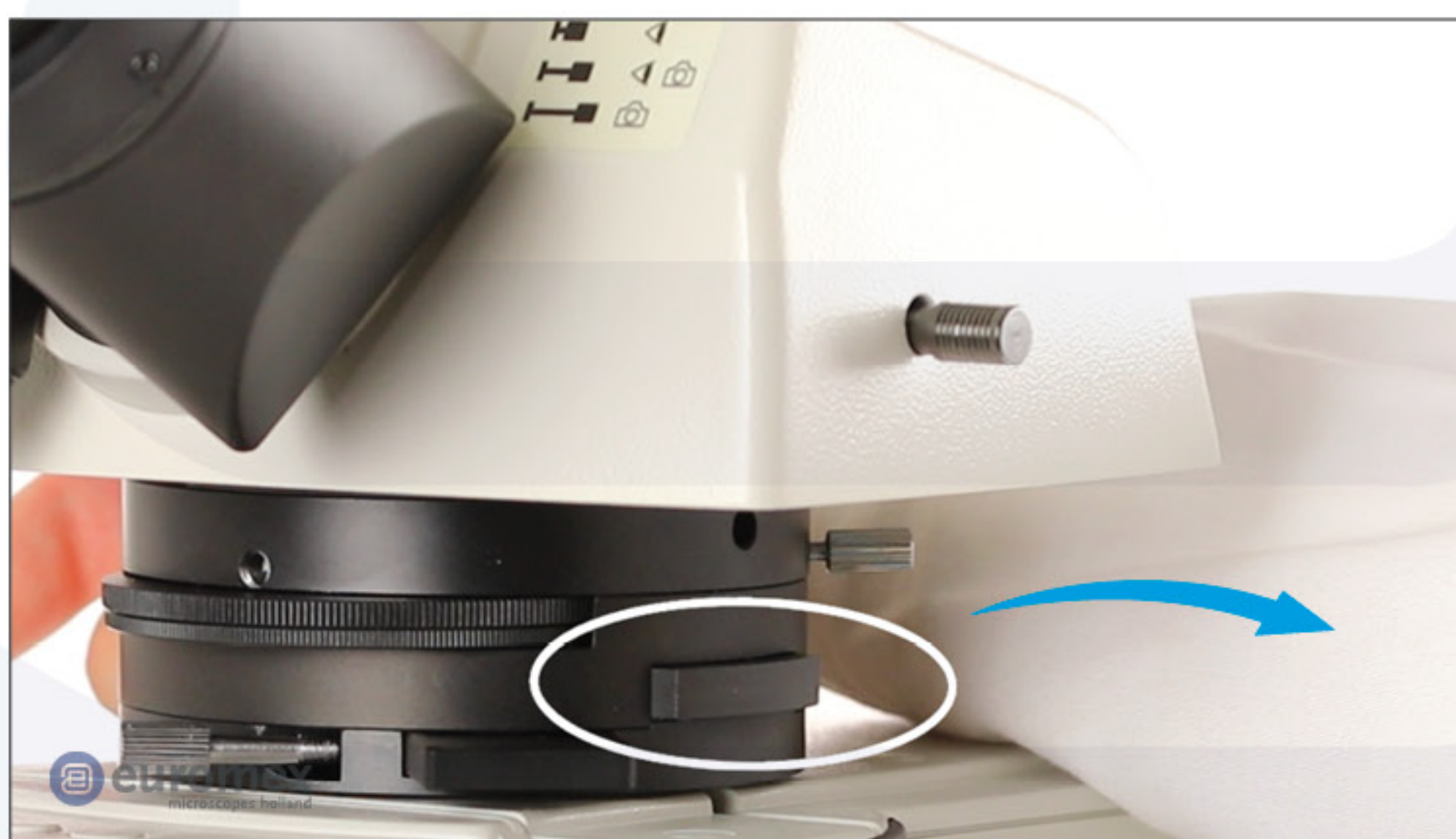
To insert the analyzer, first remove the dust protection
