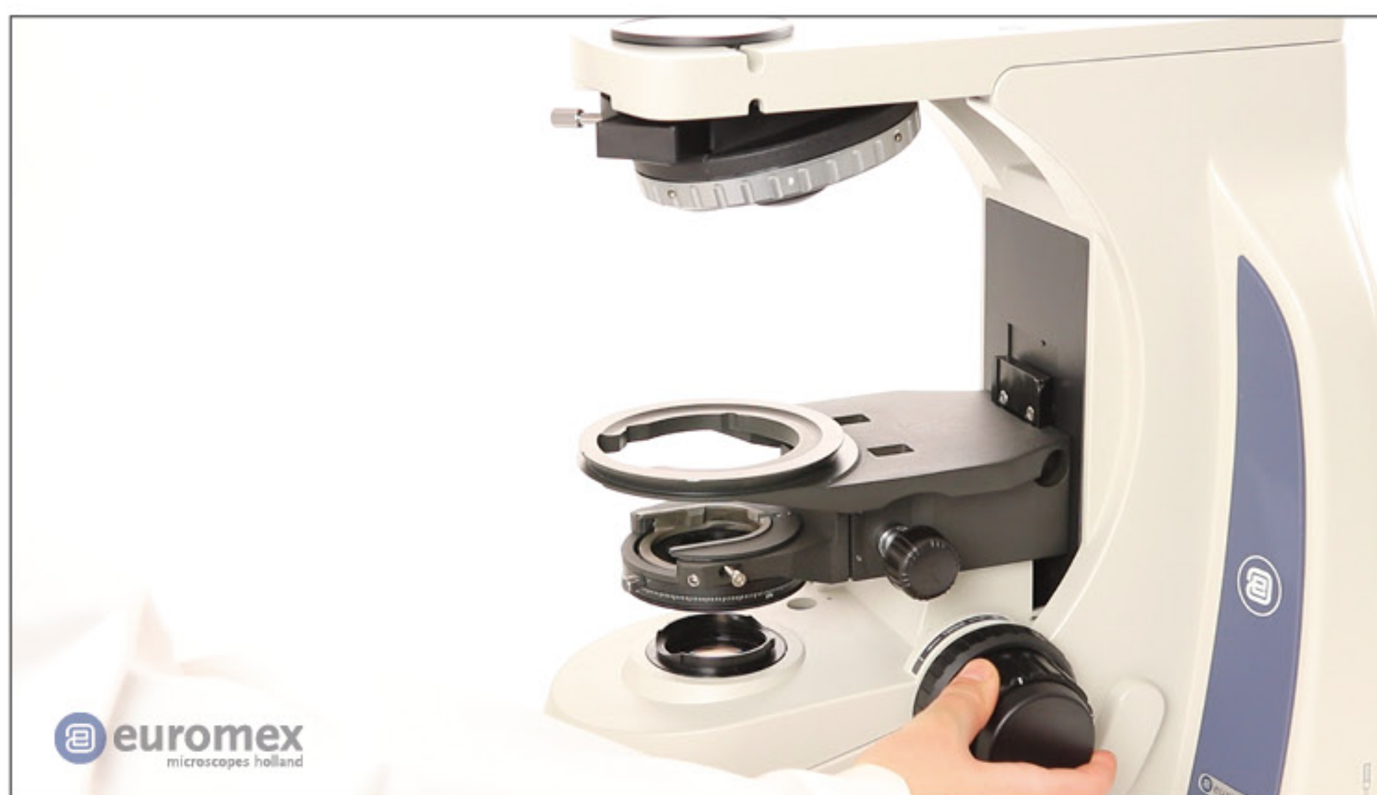
Move the stage holder to its lowest position
