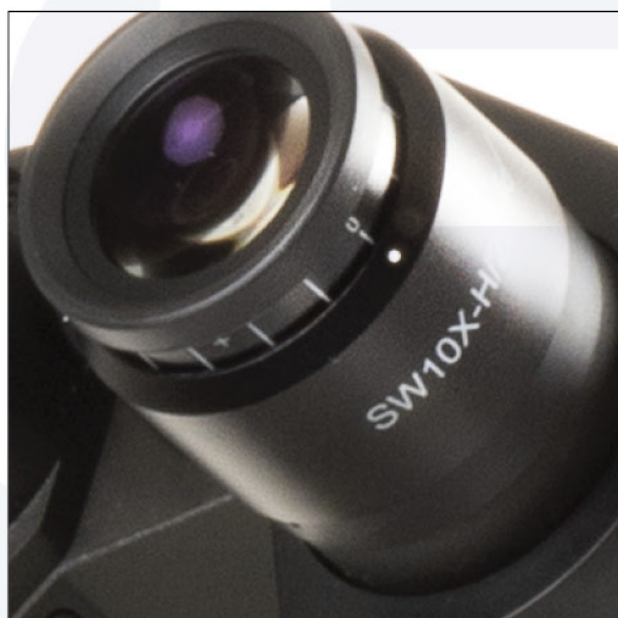
Adjustments of dioptré of a compound microscope
