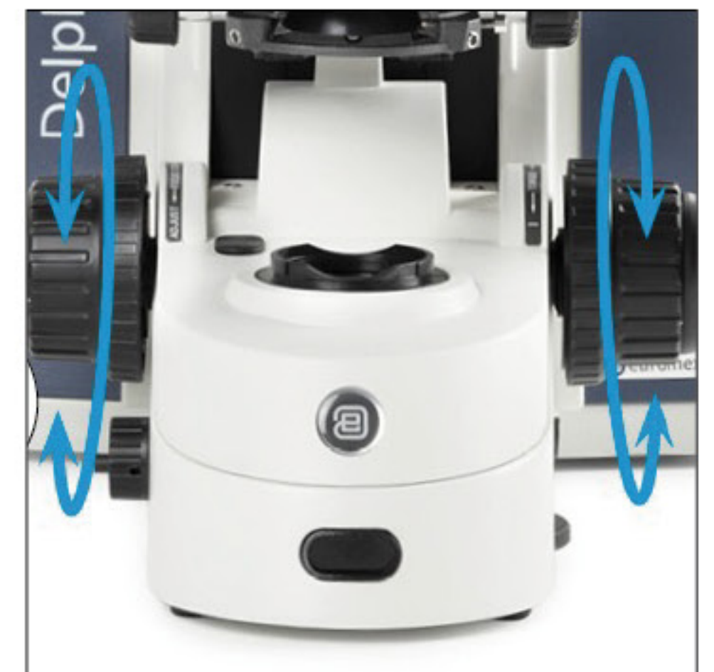
Getting the specimen in focus
