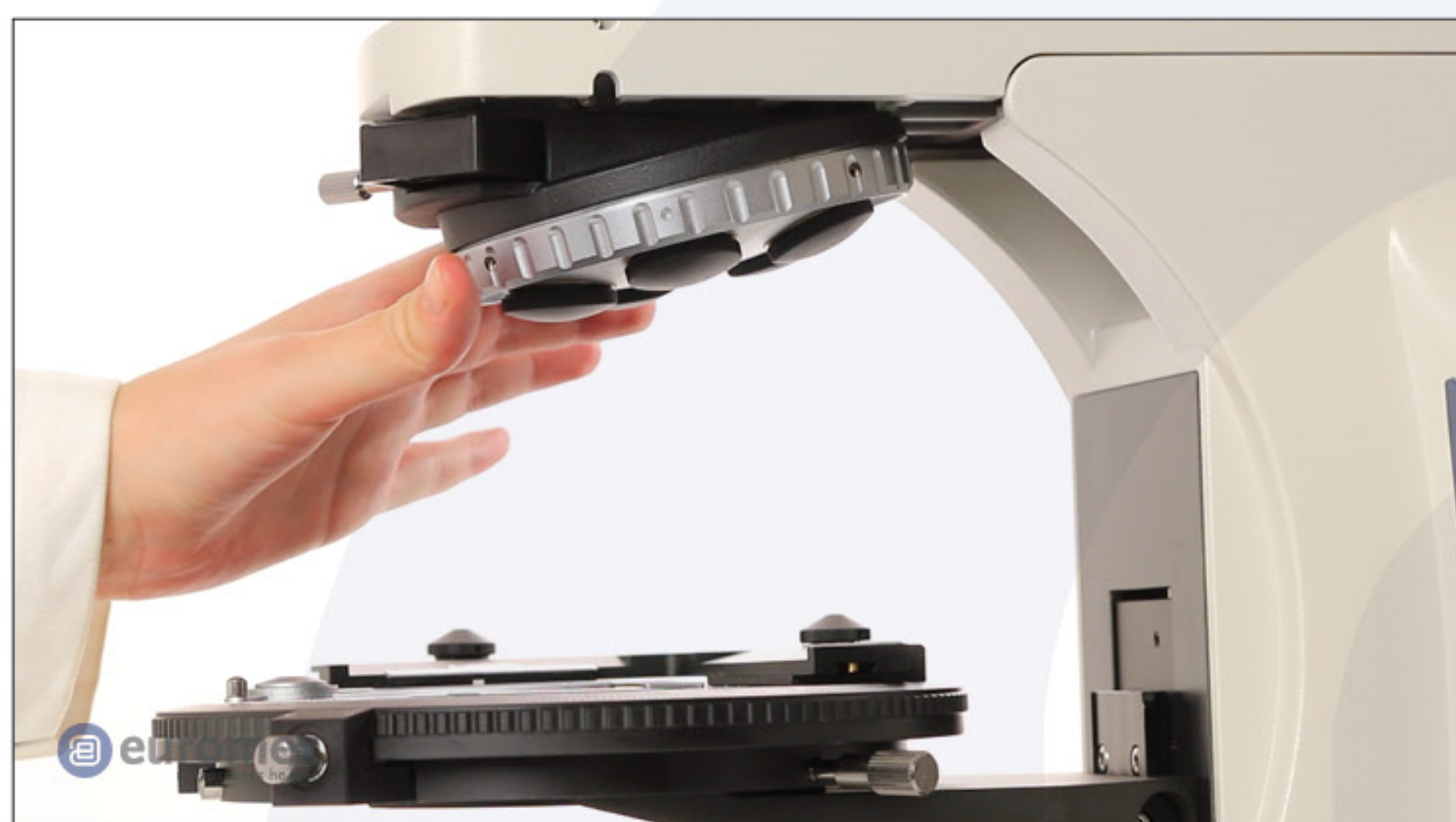
Note the indicated position (indentation) where the 5× objective should be installed
