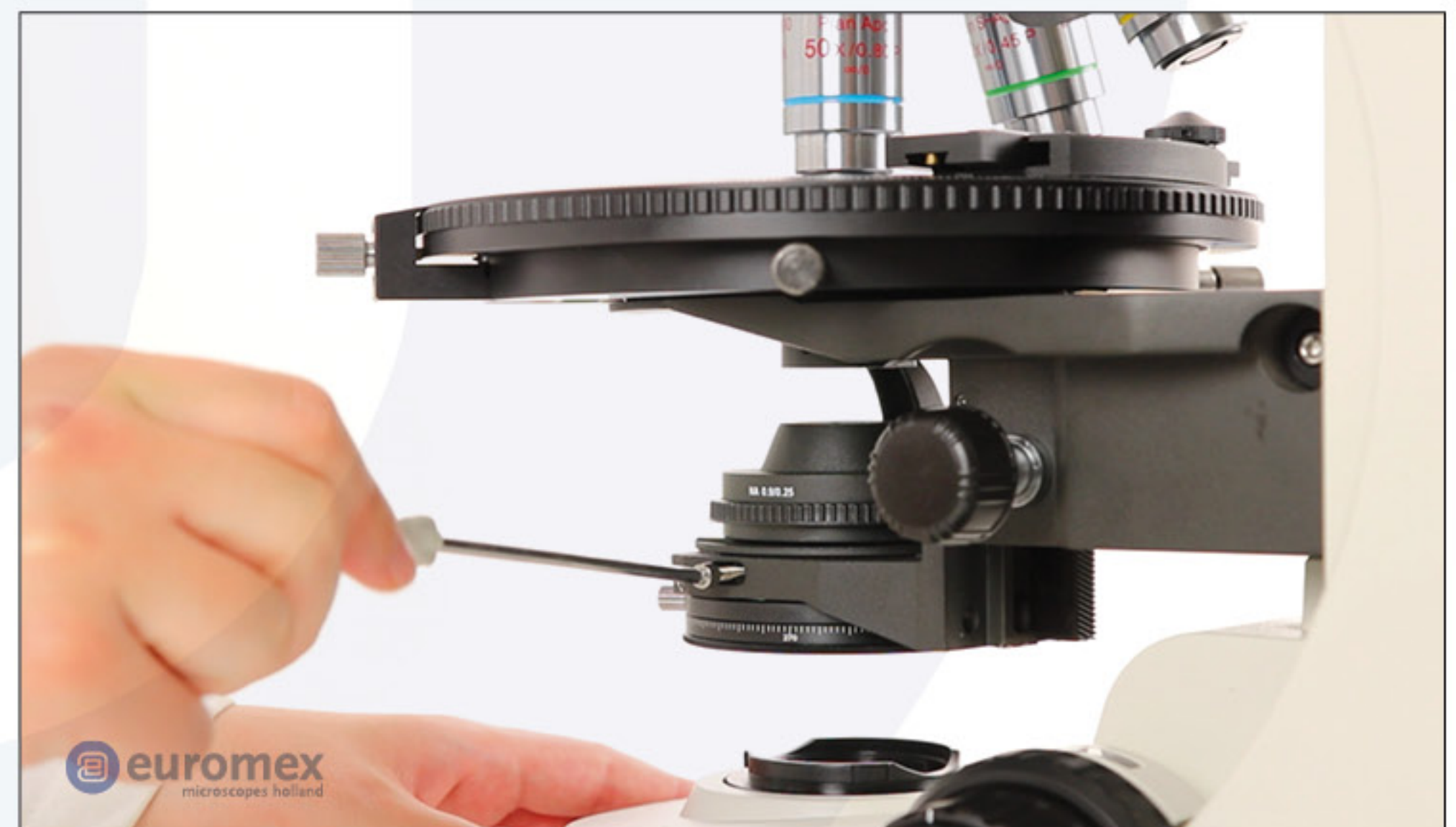
Secure the condenser in place by tightening the screw
