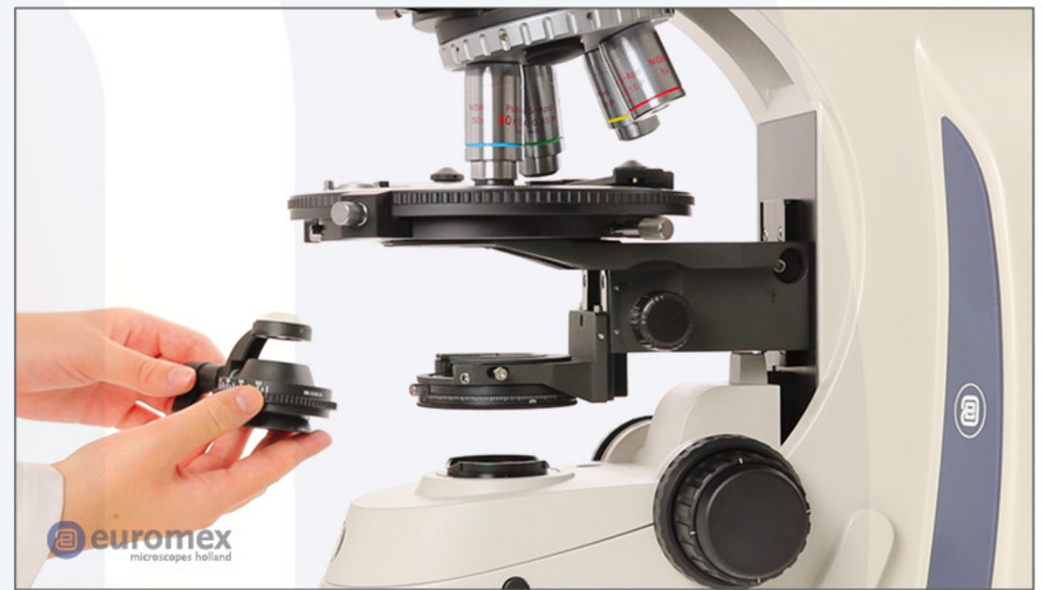
Insert the condenser into the condenser holder
