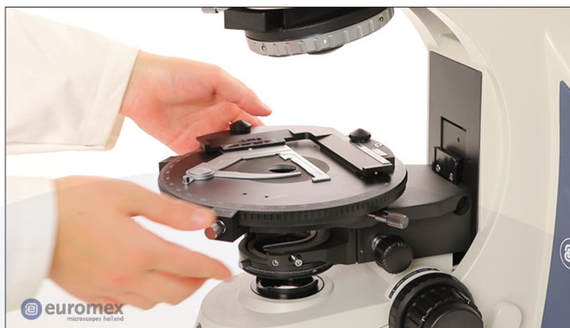
Secure the stage in place
