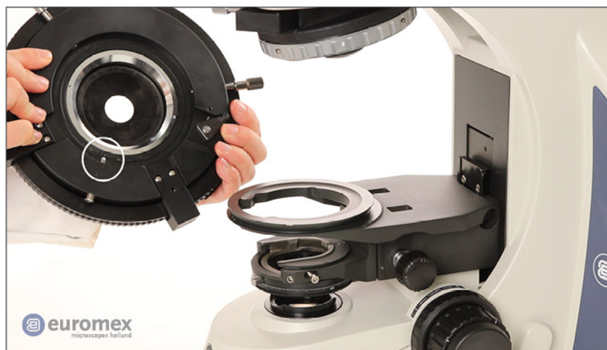
Before attaching the stage, note the position of the spring-loaded screw and where it should be placed
